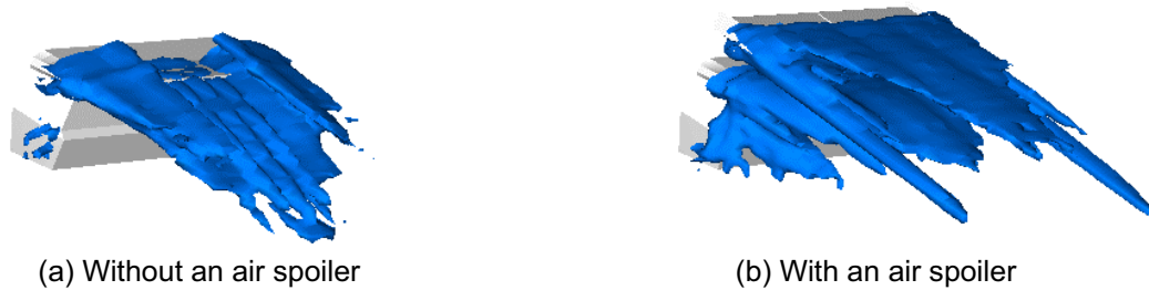
Fig. 5. Isosurfaces of the absolute vorticity |\omega| reconstructed from the x - y and z - x plane data.
